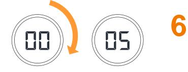
After closing the lid(cap), turn the circular panel in front of the centrifuge clockwise to set to 5 (5 minutes. increment by minute). It works after 5 seconds after setting the time. You can increase the time further as needed. X Reset: On/off with the click of a button X Pause: Open a below drawer or lid(cap)
