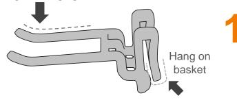
As shown in the left image, there are hooks provided with the centrifuge. The hooks are for fixing the Direct Aligners to the basket.
