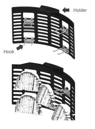
Install the hooks as shown in the image below. Mount the holder securely to the basket. Please check if the basket is correctly installed in the grooves at the bottom of the centrifuge.
