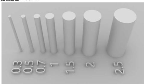
Minimum Hole Diameter, X-Y plane
