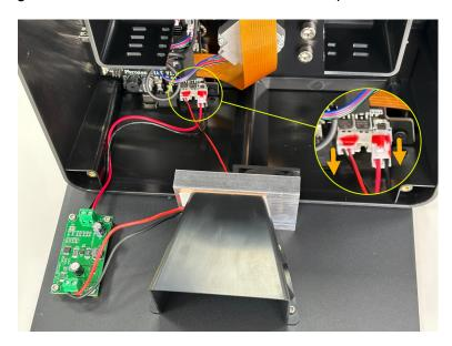
Step 6: To disconnect the LCD ribbon cable, open the cable clip and detach it (see the picture 1 2 below).
