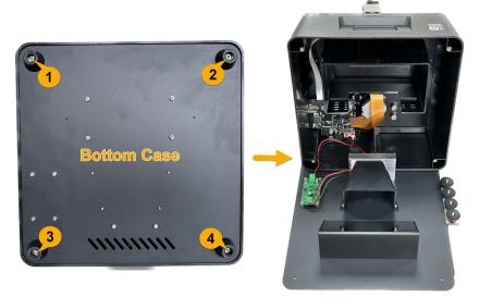
Step 5: Unplug the LED connector and fan connector and put the bottom case aside.
