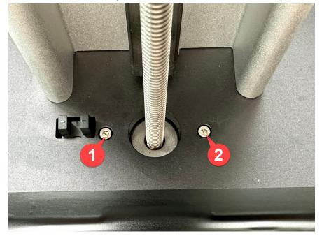
**Step 9:** Turn the Z-axis counterclockwise until it becomes loose while holding the T-plate with the other hand.
