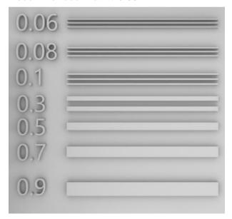
Minimum Engraved Detail Width, X-Y plane
