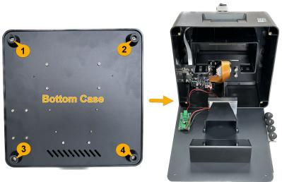
**Step 4:** Disconnect all cables/ wires (see the below picture) that are linked to the mainboard.
